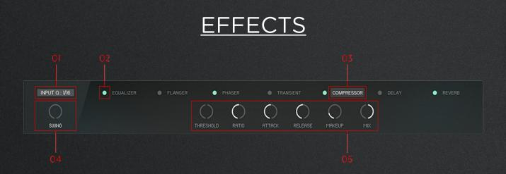
**O1 INPUT Q** - Activate and select the input Q timing in this dropdown menu.
